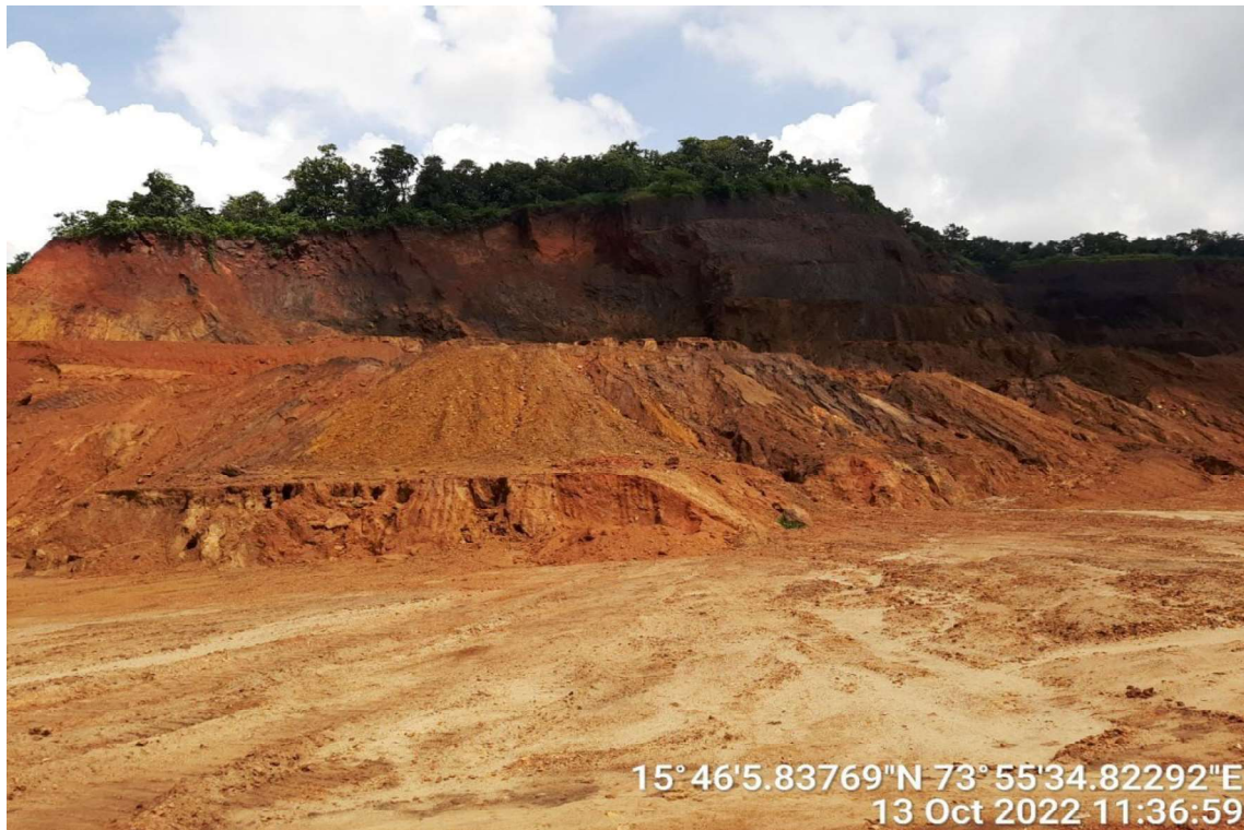
Photograph-2: Earlier mine pit, scrapped and leveled with overburden.
