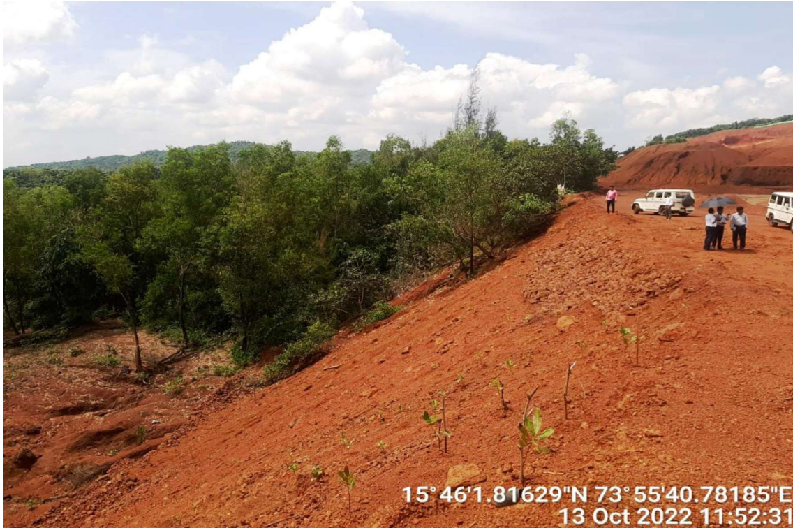
Photograph-5: Mine boundary wall augmented with overburden and plantation of cashew saplings.
